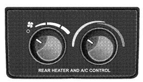
The rear compartment control uses two rotary knobs: one for the temperature control and the other for the fan speed control. The mode for the rear air conditioning and heating system is always controlled by the front control unit. Fan and temperature can be controlled from the front control unit or the rear control unit.
